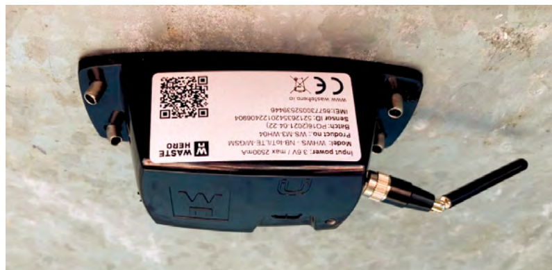
Figure 10: GSM network container filling sensor Source: Kežmarok (2022c)
